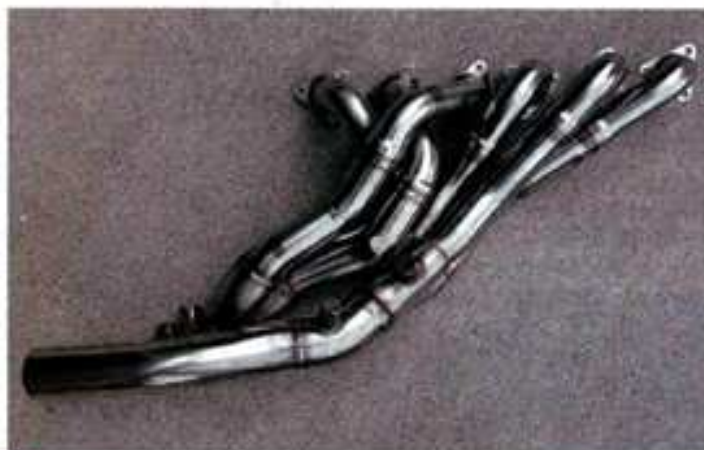
■ The Supersprint arrangement replaces the entire stock system with a set of patented stepped headers, one pair of metallic race cats, an X-pipe and a set of street or race mufflers, deleting one pair of cats and a resonator in the process.
