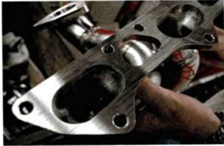
(Left) A prototype muffler showing off its muffling. (Right) Finishing the exhaust manifold port.
