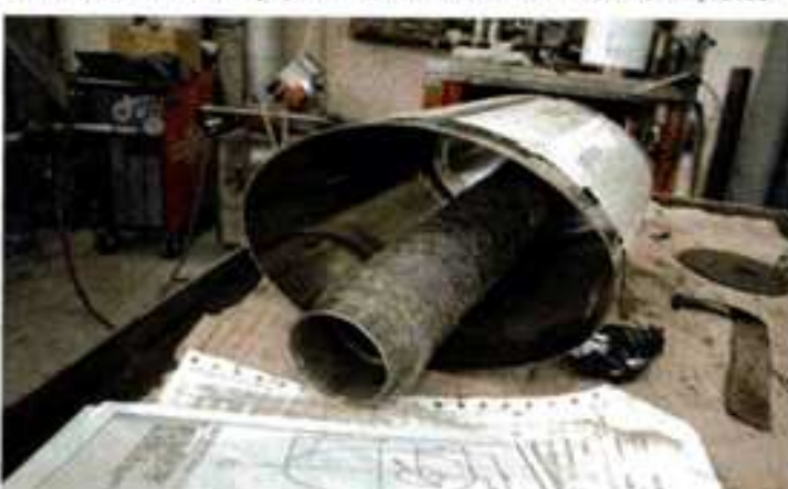
(Left) Everything stops for lunch. Even work at Supersprint's exhaust system digitizing table. (Right) A first-pass prototype muffler in the process of being built.
